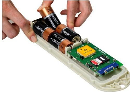
The Remora uses 4 x C-Cell batteries.
