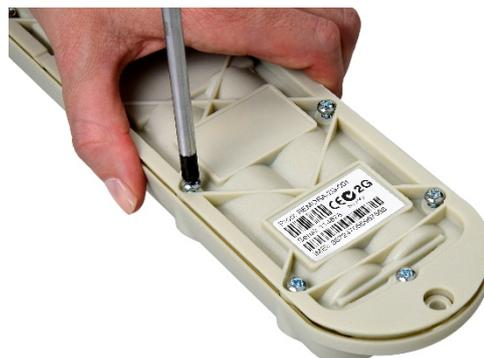
Once online, all that remains is to seal the housing. Seal the device carefully to achieve the IP67 rating.
